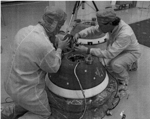
Fig. 7 Flight SRC in final integration; parachute installation.
